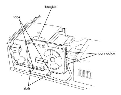
The two tabs at the bottom of the mounting plate should be just above the two slots in the computer case.
